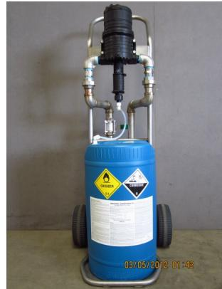
With the **SAFE T DOSE 45** this is eliminated. The worker simply rolls the cart to the location of the tank to be sanitized, hooks up the Tri Clover water line typically used to fill the tank, and opens the flow valve.
