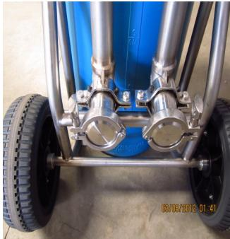
Once the operator has added the required amount of water to the tank A simple flip of the pump valve turns off the pump and rinses the line with potable water
